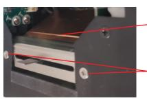
Innofader Rane 1-70-72 can be mounted in any of the 3 fader slots. For the crossfader, copper back will face inside the Rane mixer.
