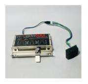
Use the mini black screws to assemble the bracket to the fader. When properly assmbled, the stem will travel freely back and forth.
