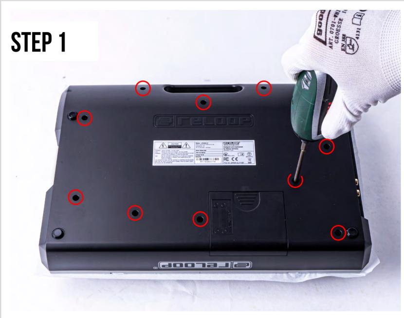
Remove all screws from the bottom housing.
